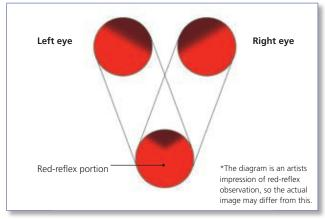
The illumination system of the OMS-90 produces a superior red-flex image for assistance in surgical procedures. As shown in the diagram, the innovative system design merges two improved field of views to produce an enhanced redreflex and unparalleled image quality.
